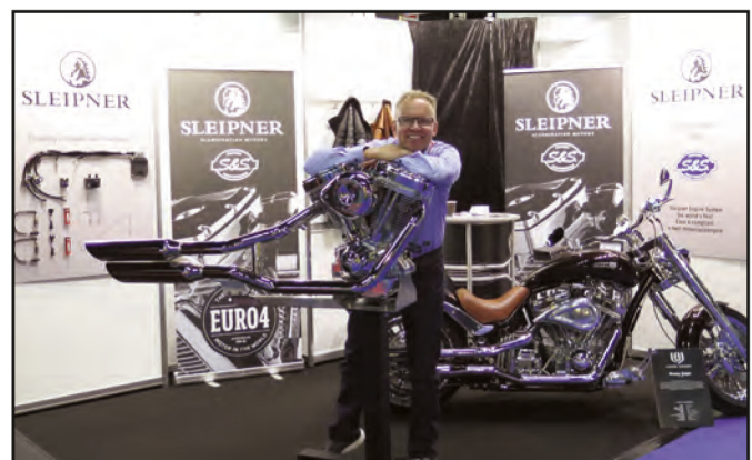
Lauge Jensen Engineering: Uffe Lauge Jensen chose INTERMOT for the debut of the EURO 4 compliant 'Sleipner' 1800cc/111" 45 degree v-twin engine program co-developed with S&S Cycle. The EURO 4 emissions regulations come into effect in January 2016 and with a v-twin builder package that includes compliant catalytic converter equipped exhausts, this is the first aftermarket EURO 4 compliant engine available; www.laugejensen.dk
